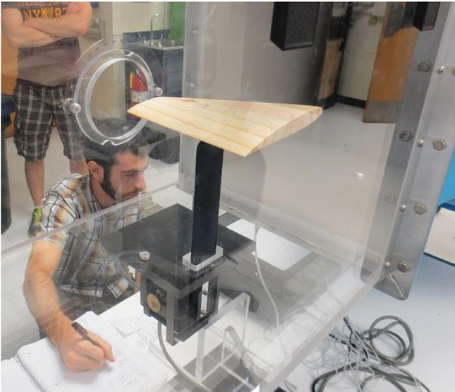
Figure 3. Hydrofoil mounted in the wind tunnel
