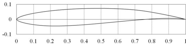
Figure 2. Eppler 817 cross section used to design the hydrofoils tested on the prototype
