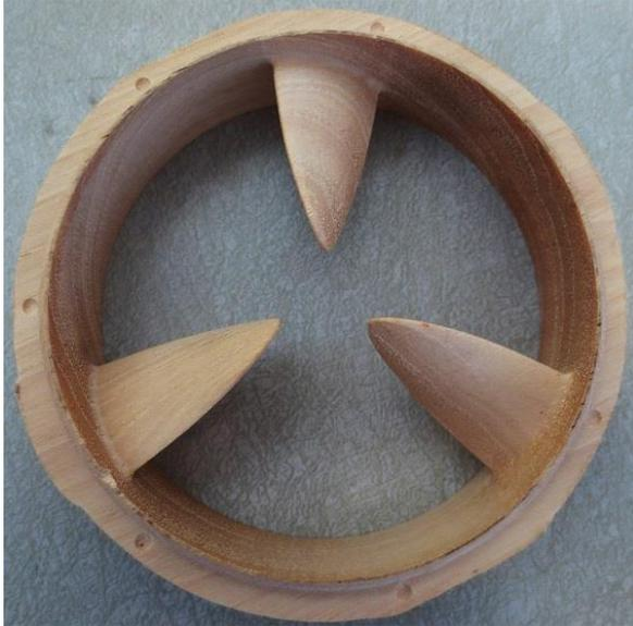
Figure 8. Hubless propeller designed and manufactured for PropaGator 2
