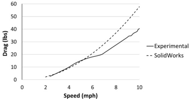
Figure 5. Drag test and simulation results
