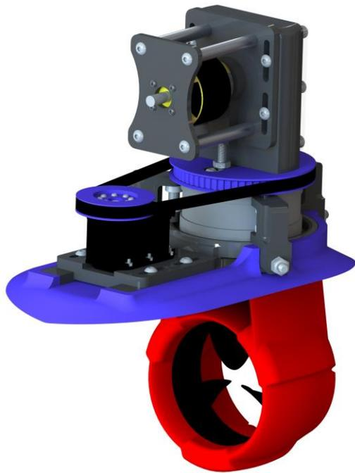
Figure 7. Assembly of PropaGator 2's propulsion system
