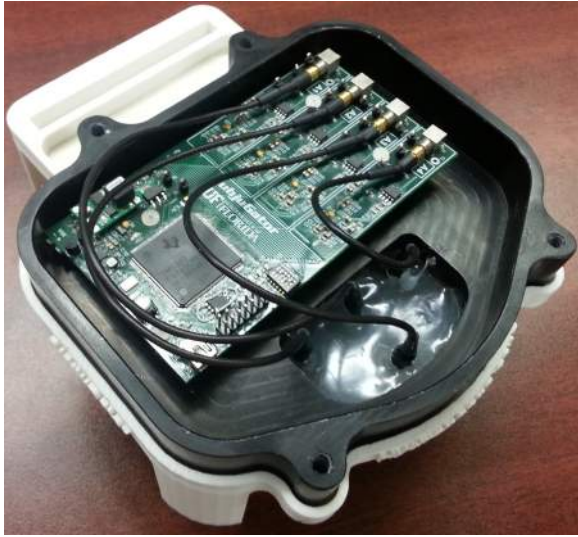
Figure 11. Passive sonar amplification and processing hardware
