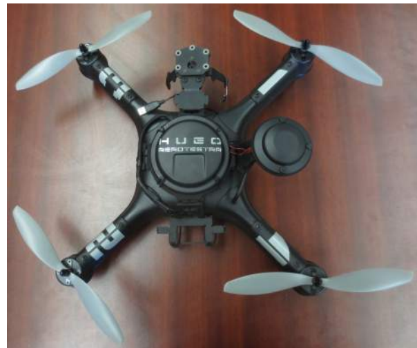
Figure 9. HUGO, a waterproof quadcopter used by PropaGator 2
