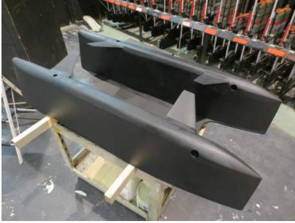
Figure 4. Underside of the wooden prototype hull featuring hydrofoils
